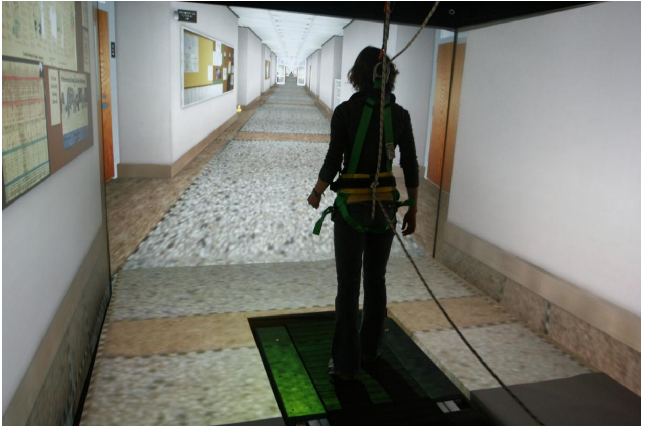
Figure B1. Large-screen virtual environment set-up with treadmill and harness.
